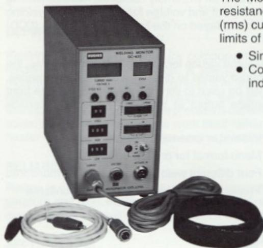
The Model QC-432 welding monitor will monitor peak voltages across the interface of a resistance weld or peak current through the weld. The QC-432 will also display root mean square (rms) currents and the number of ac cycles with a digital liquid crystal output. Upper and lower limits of optimum welding current or voltage can be preset with digital thumbwheel switches.
